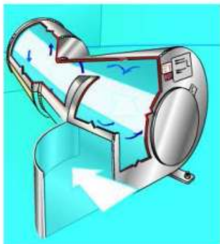
High storm event - central vortex created which displaces water into pond to control discharge rates.
